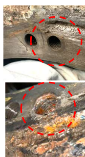
Example of Corrosion on the Hull Mounting Surface
